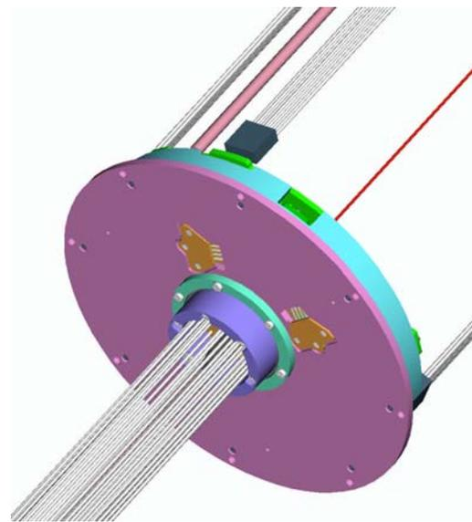
**Figure 14: Solid Model of CETS Slip Ring**
