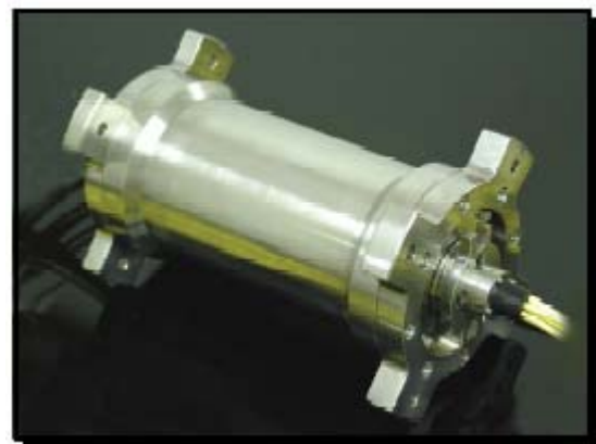
Figure 11(b): Multi-Channel FORJ with common optical path
