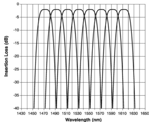
However in the past few years coarse wave division multiplexing (CWDM) has become commercially available. This technology can optimally provide around 8 channels with around 20 nm wavelength spacing. Figure 20 illustrates the wavelength separation for an 8 channel CWDM multiplexer.
