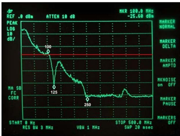
**Figure 4: Frequency Spectrum of 100 BASE Ethernet**
