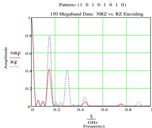
**Figure 3: 150 Mhz square wave Fourier components**
