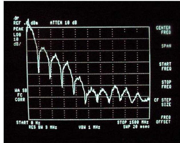
**Figure 5: Frequency Spectrum of 150 Mbps Hotlink**
