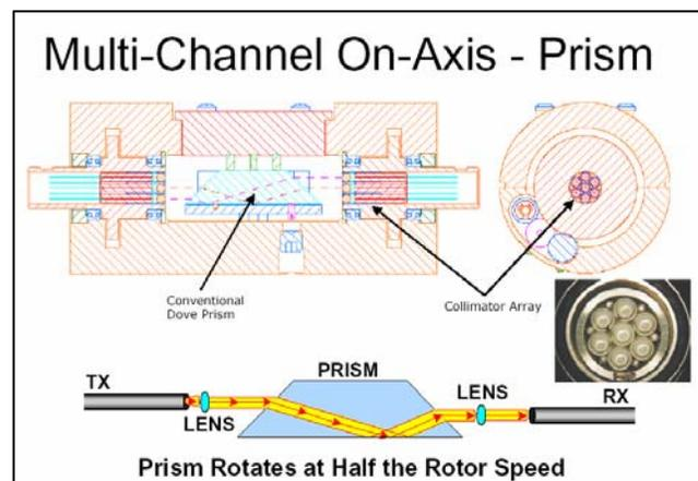
**Figure 12: Dove Prism as a common optical path**
