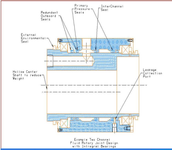
**Figure 2. Fluid Rotary Joint with Standard Lip Seal Design**
