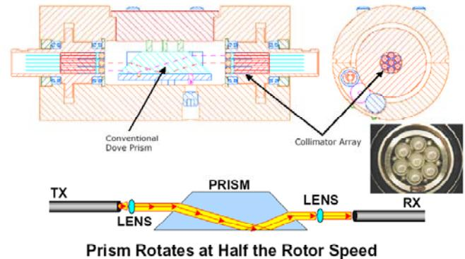
**Figure 4. Multichannel On-axis FORJ**
