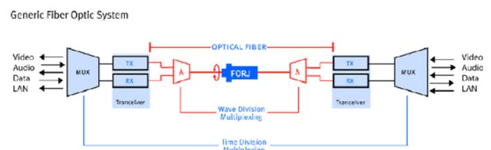
**Figure 6. Multiplexing Solution for Multiple Signal Paths with Bidirectional Light Transmission**
