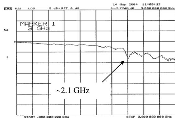
**Figure 3. Insertion Loss vs. Frequency on Broadband Slip Ring Design**
