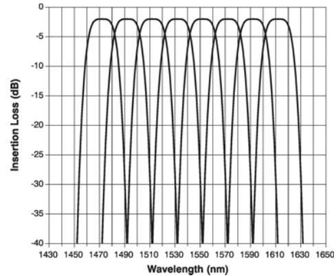
**Figure 7. Typical Wavelength Division of 8-channel Coarse Wave Division Multiplexing (CWDM)**
