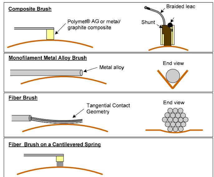
**Figure 1. Comparison of Sliding Contact Technologies**
